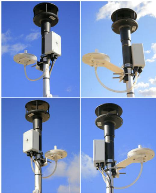
**Figure 13:** Different angles display the instrument mast and sensors post-tornado. The instrumentation was cleaned externally to remove soil impurities. Photos by Bob Fritchie.
