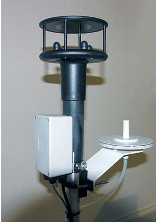
**Figure 6:** Top of the instrument mast containing the Gill WindSonic anemometer, Vaisala pressure sensor (inside enclosure), and R.M. Young static pressure head. Photo by Eric Nguyen.
