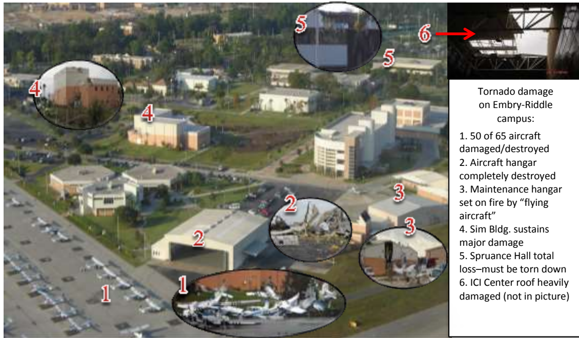
Figure 4: Photograph of Embry-Riddle campus with locations of worst damage shown by markers numbered 1–5. Each location has an associated inset picture showing the damage. The ICI Center is located to the east of Spruance Hall (marked '5') and not included in the picture; however, the roof damage is shown by the picture marked '6' in upper right corner of figure.
